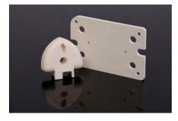
Syntactic foams are a unique combination of hollow spheres, a resin matrix, and other additives. When combined and processed properly, the constituents form a lightweight homogeneous material having high compressive and hydrostatic strengths. This yields a product able to withstand the extreme hydrostatic pressures experienced by today's manned and unmanned subsea vehicles.
